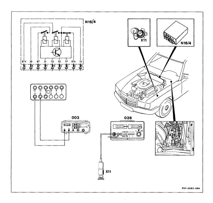
N16/4 Fuel pump relay with kickdown cut-out X26 Connector, interior/engine
