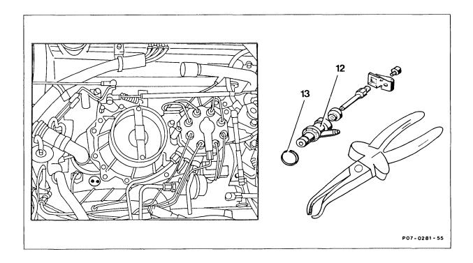
Ground cable on control bearing pedestal . . . . rear left, disconnect, reconnect. Shaped hose for auxiliary air . . . . . remove, mount.
