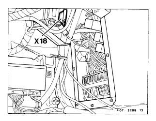
Model 126, pull off fuel pump relay (N 16/4). Bridge jacks 7 and 8 (terminals 30 and 87).
