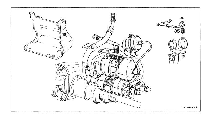
Protective cover (10) ..... unscrew, screw on. Rubber buffer (35) ..... remove, reinstall.
