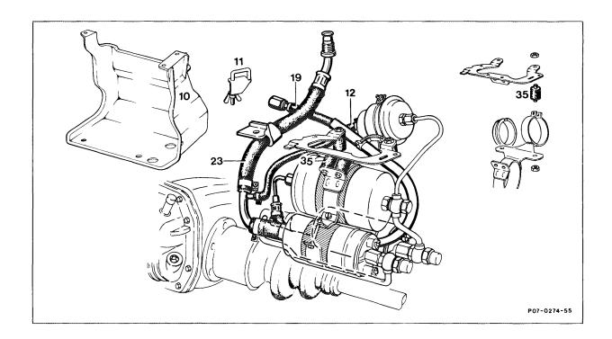
Pressure in fuel tank ...... release by opening screw cap. Battery ..... disconnect, reconnect. Protective box (10) ..... unscrew, screw on. Electrical wiring ..... disconnect, reconnect. Fuel suction and delivery hoses (19 and 23) .... pinch with clamp (11) and remove. Special tool 000 589 40 37 00 Fuel suction, leak-off and delivery hoses (12, 19 and 23) ..... unscrew, screw on. Rubber buffer (35) ...... remove, reinstall.
