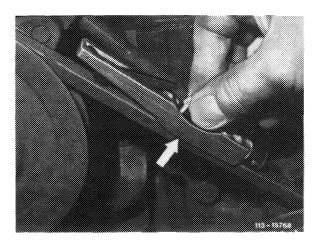
5 Read adjusting value on intersection of indicating arm and upper scale (KG scale, arrow).
