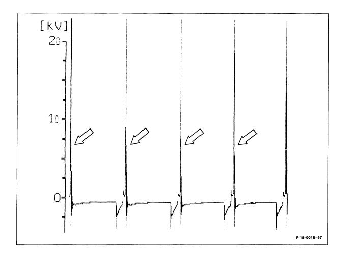
15. Ignition voltage < 8 kV at terminal 4
