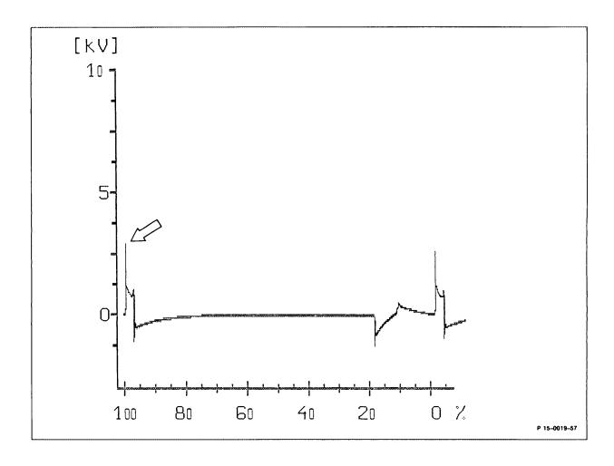
16. Ignition voltage < 6 kV at single cylinder.
