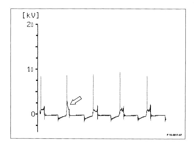
14. Higher spark voltage > 1.5 kV at all cylinders
