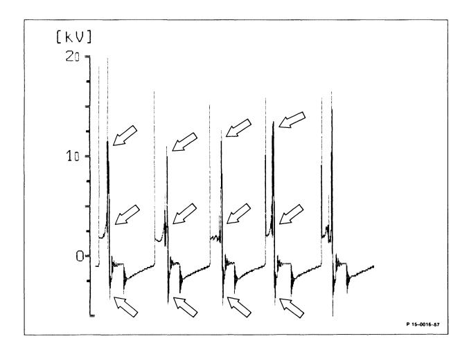
13. Higher spark voltage > 1.5 kV at single cylinder
