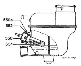
Coolant level transmitter 550a 551 Locking ring Float
