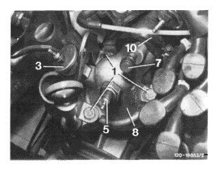
Instead of vent hose (arrow) by way of which the cooling system has been continuously and automatically vented during filling operation and also during operation of engine, the vent screw (7) has been used up to August 1981. This screw must be opened for venting when filling the cooling system. When using this vent screw, no automatic, continuous venting of cooling system will occur.
