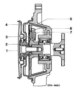
Starting at a coolant temperature of approx. 105 °C, the bimetallic strip (1) is heated by the air flowing through the radiator so that it will change its shape and arch in an outward direction. The spring plate (3) can now clear the transfer bore (5), as a result of which the circulation of the viscous oil is established and the viscofan clutch is engaged.
