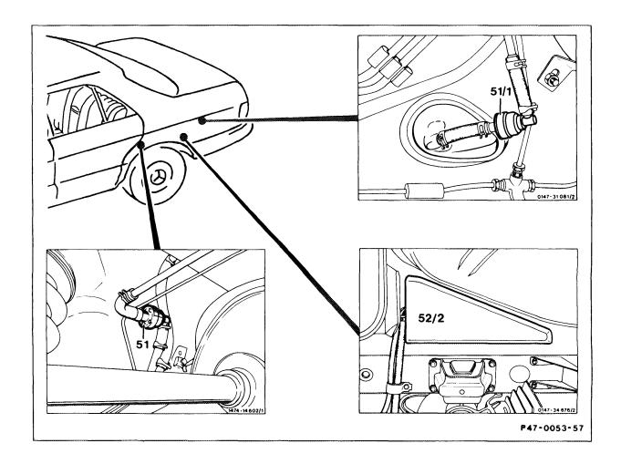
51 Vent valve Model 107 51/1 Vent valve Model 126 52/2 not used
