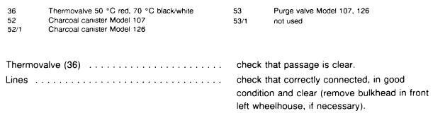
approx. 80 °C. detach line at right angled connection fitting in left side of engine compartment. Slowly increase engine speed to 3000 rpm. No suction action at idle speed. Suction action commences as engine speed increases.
