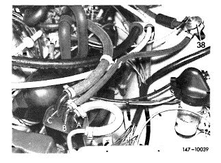
• On vehicles with fuel evaporation system, check all parts for condition and leaks.
