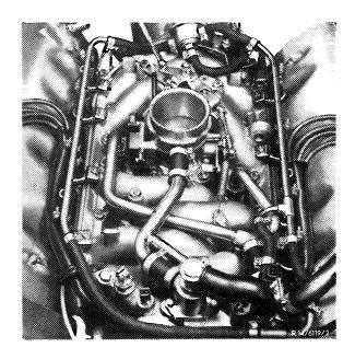
• On vehicles with electronically controlled gasoline injection system, be sure to check fuel hoses in engine compartment for leaks and condition.
