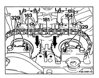
NOTE: If both camshafts are taken out at the same time, mark each for later identification because they are identical.
