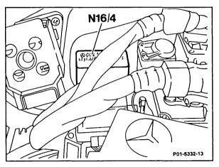
Connect once clamp of remote starter switch to the battery positive terminal.
