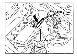
Disconnect connector (X27) from plug connector 50. Connect plug from adapter cable (01) 124 589 36 63 00.
