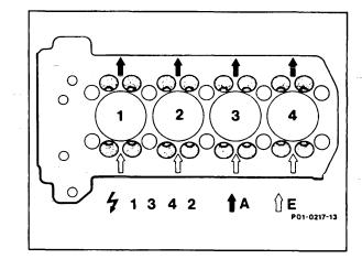
Measure valve clearance between bucket tappet and cam base circle (arrows).
