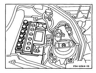
Check fluid level in filler opening of cells and, if necessary, add fluid up to the inner marking.
