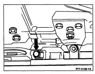
Replace damaged sliding jaws.
