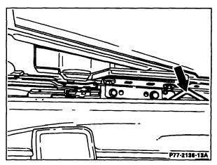
Insert sunroof panel from above, start nuts, preload sunroof panel using tool 124 589 00 37 00 and tighten nuts.
