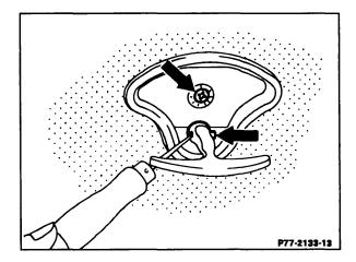
Open sunroof completely and remove sliding rails on left and right side.
