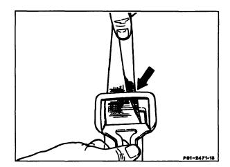
Note: If customer complains that belt does not roll up neatly, check whether belt is guided back manually as specified or whether it is twisted 180° behind panel caused by improper handling. Remove panel for this purpose.
