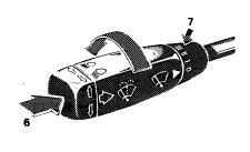
To signal minor directional changes of the vehicle, such as changing lanes on a highway, move combination switch to the point of resistance only and hold it there.
