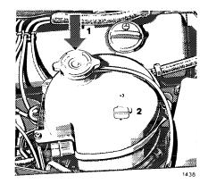
1 Coolant reservoir cap2 Marking for coolant level
