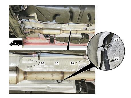
26 Remove the heat shield (25).
