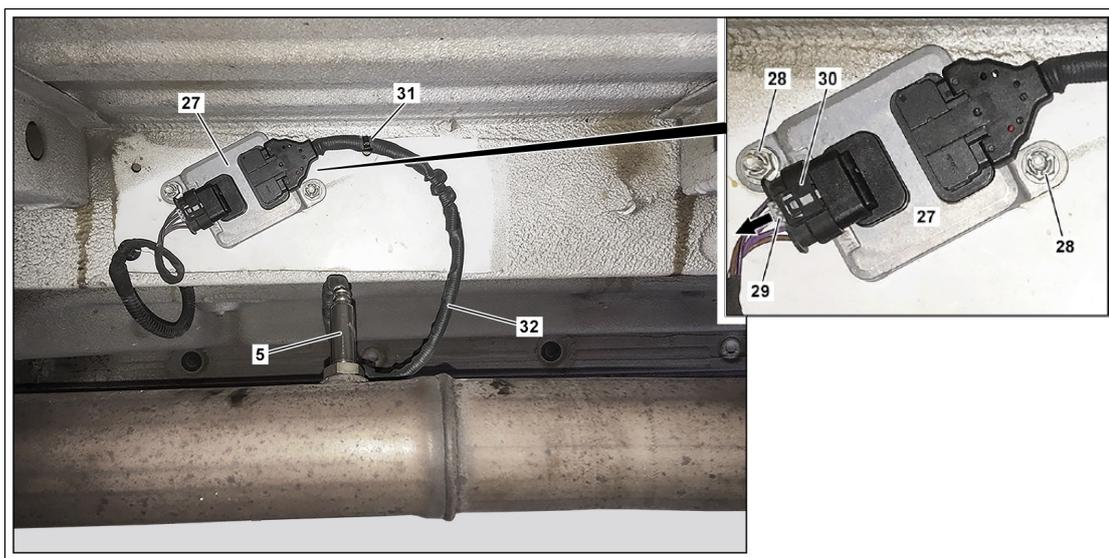
33 Disconnect the electrical plug connection (30) at the NO<sub>x</sub> sensor control unit downstream of the SCR catalytic converter (27).
