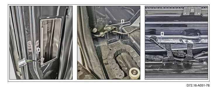
8 Closing assist motor electrical wiring harness
